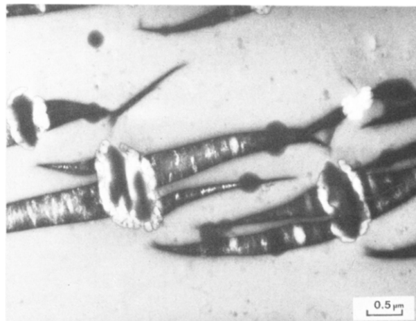
Figure 9. Electron micrograph of a stressed film of ABS cast from ethyl acetate and stained first with \text{OsO}_4 and then with \text{RuO}_4 vapor.
