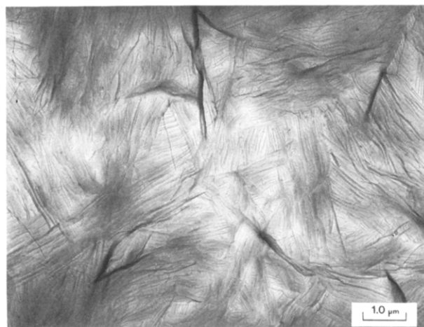
Figure 13. Electron micrograph of an unstained thin film of HDPE exposed directly to the electron beam.
